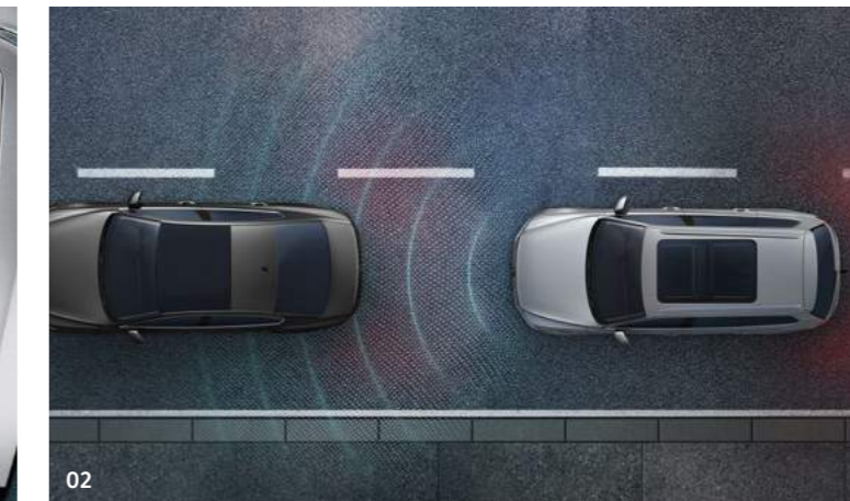
02 Adaptive Cruise Control (ACC), including Front Assist radar sensor controlled distance monitoring system, City emergency braking system, cruise control and speed limiter offers you intelligent control of your driving speed by automatically adjusting acceleration and braking. Whether around town or on the motorway, the system will adjust your speed to that of the vehicle in front, keep your specified distance, warn if you are approaching too fast and, in an emergency situation, generate enough braking force to try to reduce the severity of a collision or possibly even prevent the collision entirely. Image shown is for illustration purposes only and may not necessarily reflect UK specification.
