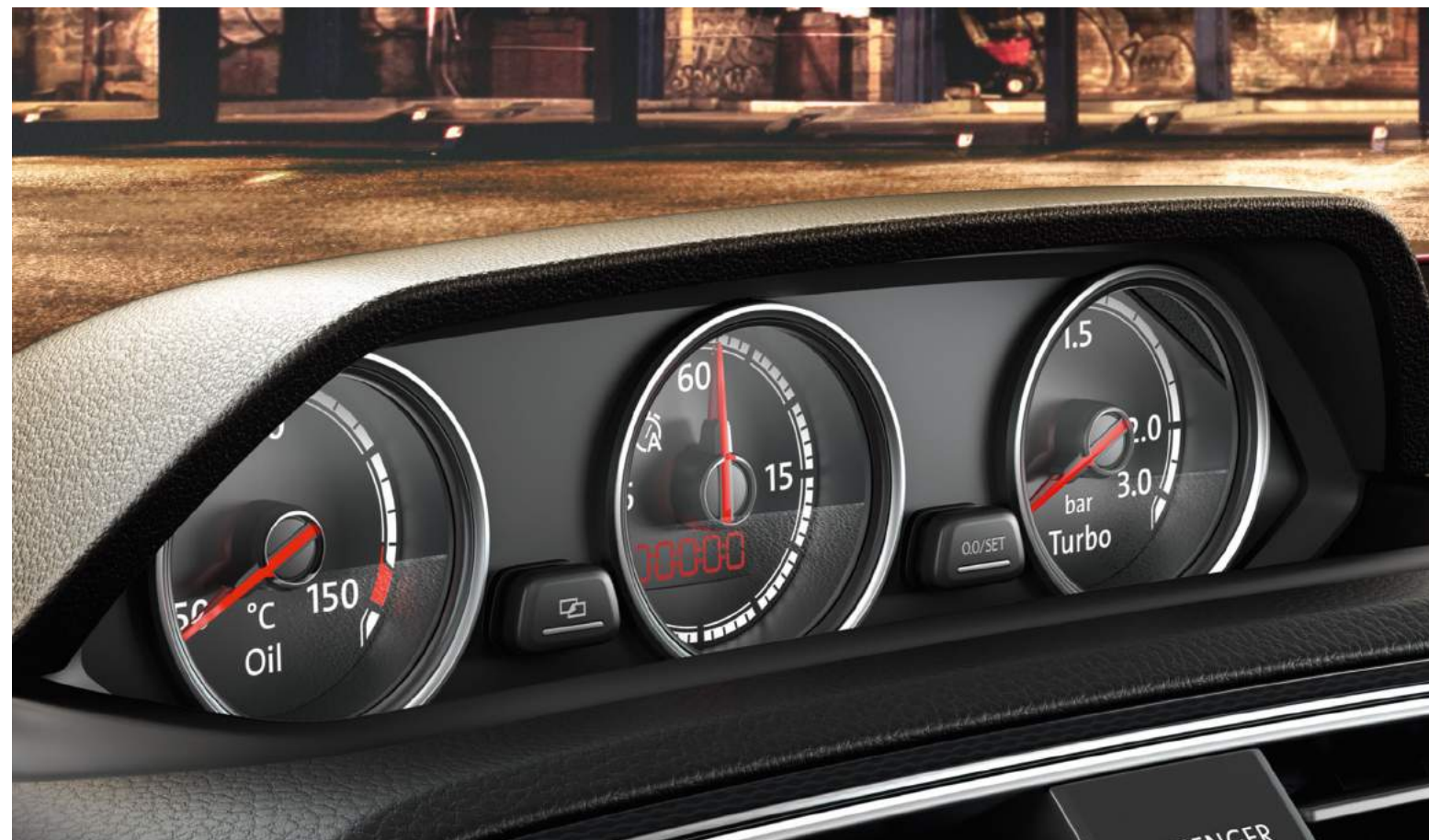
The stylish sports instrument dials above the centre console pays homage to the original 1974 model, with gauges for turbo boost pressure, oil temperature as well as a stopwatch to measure journey times.
