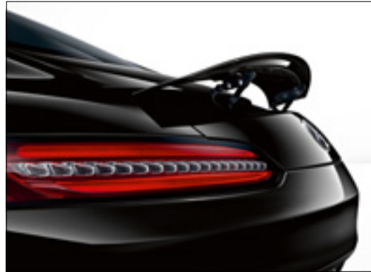
Rear aerofoil – electrically extending
