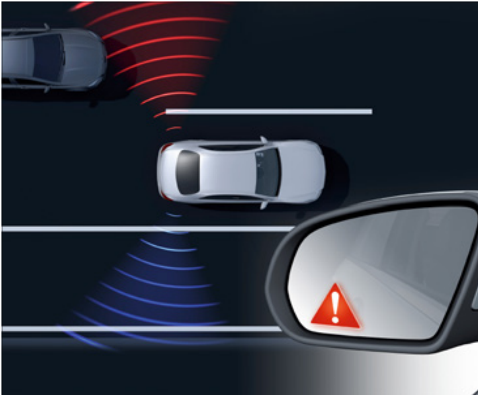
The Lane Tracking package: Active Lane Keeping Assist and Blind Spot Assist
