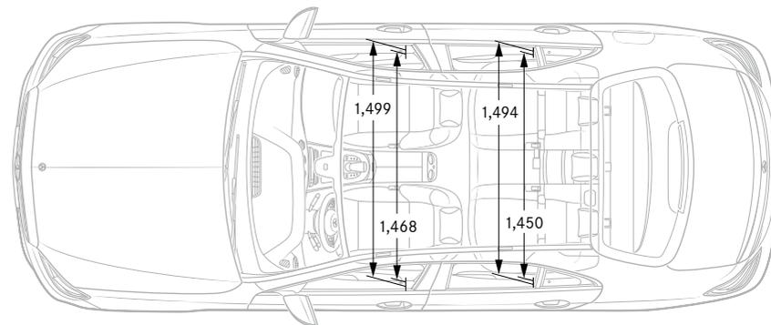
All measurements in millimetres. The dimensions are mean values and apply to standard-specification, unladen vehicles. Please note that wheels shown do not form part of standard UK specification
