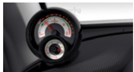
Dashboard instrument (battery charge status and power indicator)
