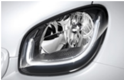
Headlamps with LED light guide: H4 halogen headlamps with Welcome-Function, fibre optic daytime running lamps, and direction indicators integrated into front bumper
