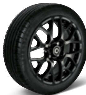
16-inch 8-Y-spoke alloy wheels (R95) painted black, with front tyres 185/50 R 16, rear tyres 205/45 R 16
