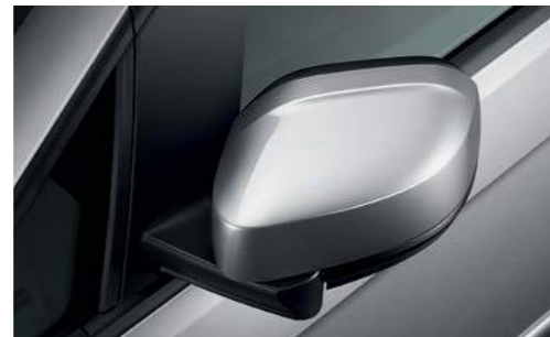
The BlueMotion's car-like aerodynamic wing mirrors. Available with optional body-coloured paint and optional electric folding function.
