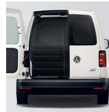
Asymmetric rear wing doors with windows. Standard on Caddy panel van.
