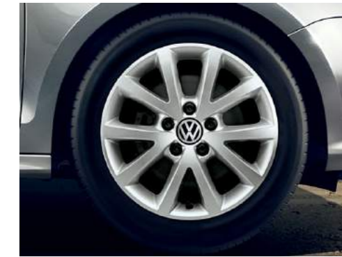
'Perth' 6J x 16" alloy wheels with 205/55 R16 low rolling resistance tyres and anti-theft wheel bolts. Optional on S and SE* models.
