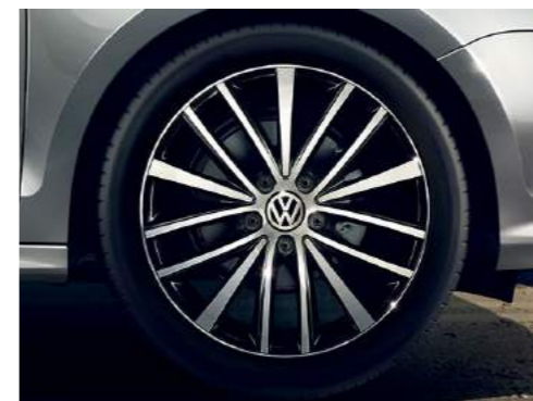
'Queensland Black' 7J x 17" alloy wheels with 225/45 R17 tyres and anti-theft wheel bolts. Optional on GT models.
