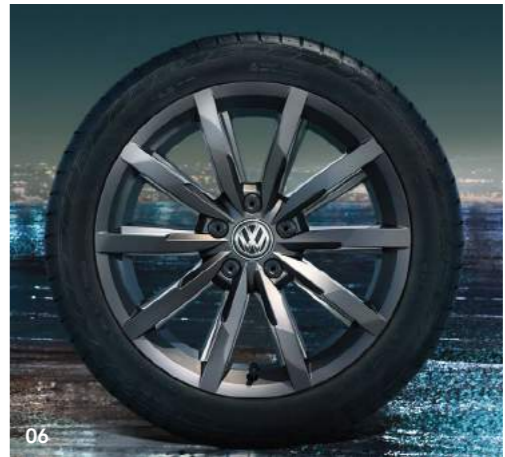
12 'Albertville' 8J x 19" alloy wheels with 245/40 R19 tyres and anti-theft wheel bolts. Optional on Alltrack models.
