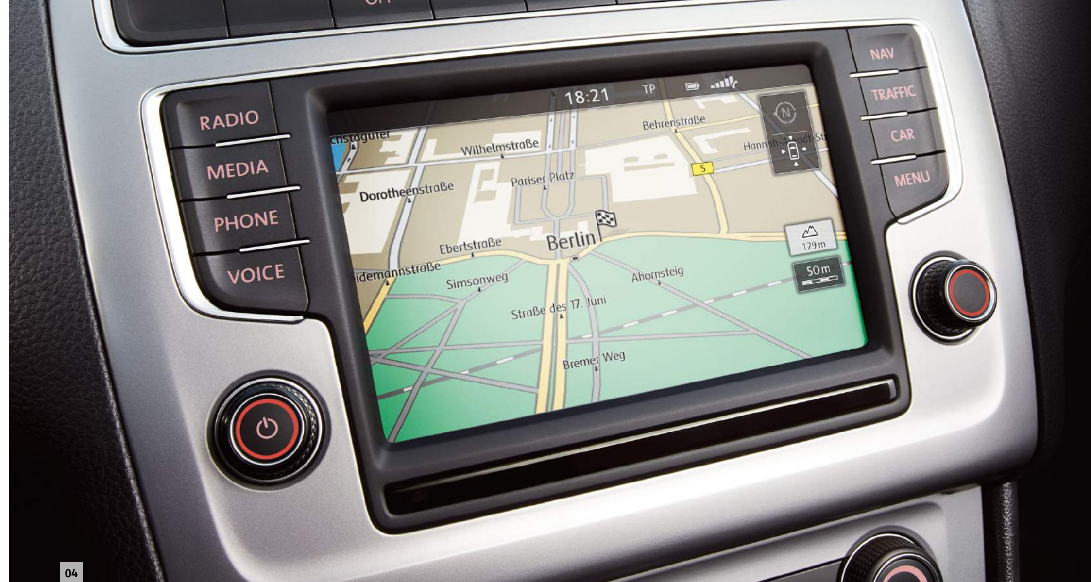
04 DISCOVER NAVIGATION TOUCH-SCREEN NAVIGATION/RADIO SYSTEM WITH CAR-NET 'GUIDE AND INFORM' 1 with 6.5 inch colour touch-screen control for navigation, CD and radio functions, is preloaded with European navigation data, 2D/2.5D map view, three calculated routes: Fast, Short and Eco, dynamic navigation based on TMC+, branded points of interest and Speed Limit Display 1 . SMS functionality (compatible Android smartphones only) – read, compose and send SMS messages using touch-screen display when your Polo is stationary. The touch-screen also features a proximity sensor which detects when your hand is approaching the screen and automatically adjusts the display, so it is ready for you to use. The navigation/radio system includes 3-years Car-Net 'Guide and Inform' 2 online access to a range of useful information such as traffic, fuel pricing, parking space availability, weather and news feeds. Online navigation software updates enable you to download the latest map data to keep you up-to-date. Optional on Match Edition models and above.
