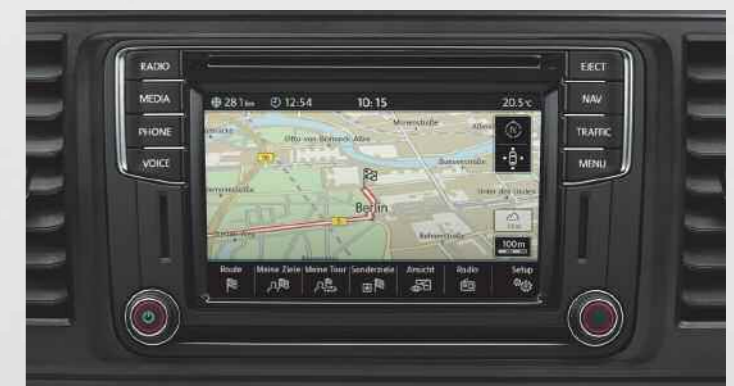
Discover Media satellite navigation system. The optional Discover Media satellite navigation system builds on the strengths of the Composition Media DAB+ radio system by adding satellite navigation and a second integrated SD card slot compatible for map data. The system includes free updates for the pre-installed European maps through Volkswagen MapCare. App-Connect is available as an option for this system.
