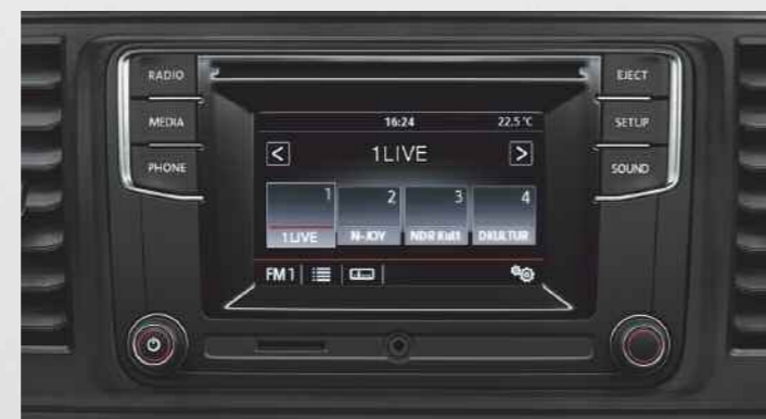
Composition Colour DAB+ radio system. Fitted as standard, the Composition Colour DAB+ radio system features a 5" TFT touch-screen colour display, USB port, Bluetooth®, SD card slot, AUX-IN interface, MP3 and WMA compatible CD drive, 4 x 20 watt output with six speakers 2 and a dual tuner with PhaseDiversity for optimum radio reception.
