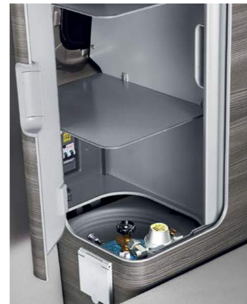
Rear cupboard with gas storage compartment for 2.8kg gas cylinder.
