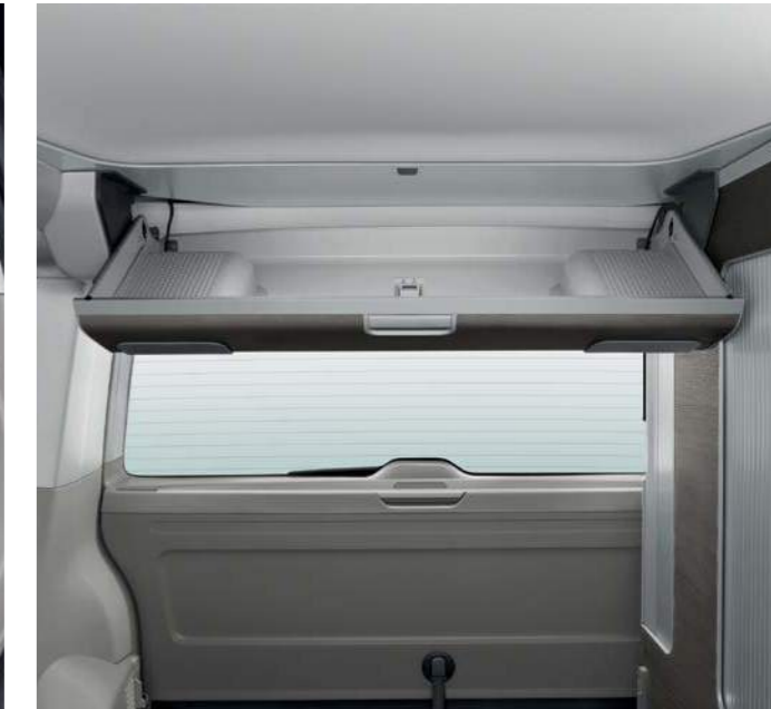
Drop-down rear compartment incorporating rear speakers.
