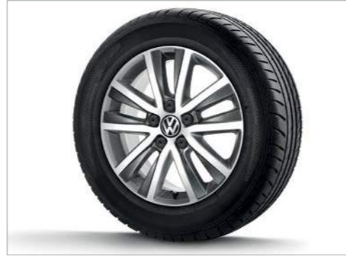
17" Cascavel Anthracite with diamond-turned surface. 17 x 7J alloy wheels with 235/55 R17 or 215/60 R17 tyres. BE OC
