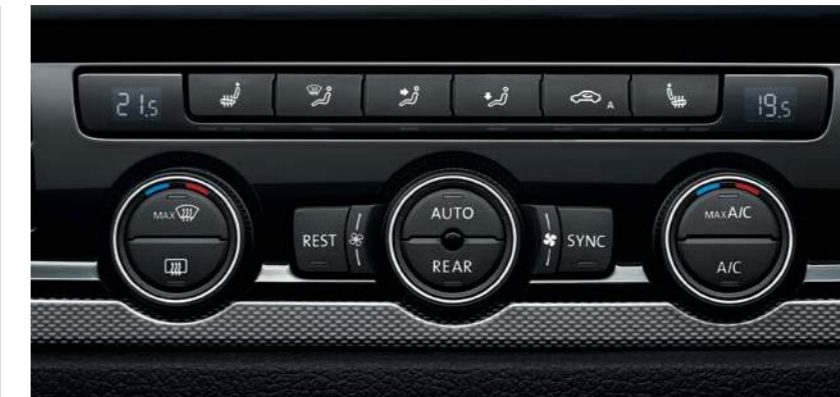
Climatronic three-zone automatic air conditioning and heated driver and front passenger seats.
