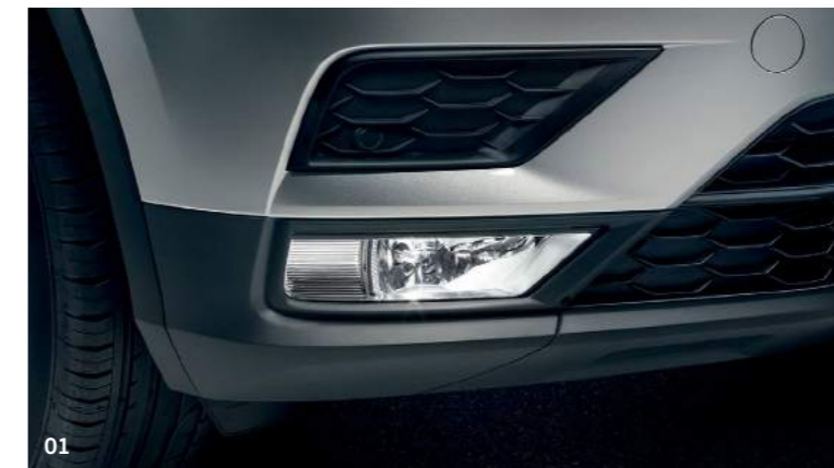
01 At crossings or junctions when travelling below 25 mph with the steering wheel turned or indicator activated, the front fog lights with static cornering function automatically switch on to illuminate the area in the direction the Tiguan is turning.
