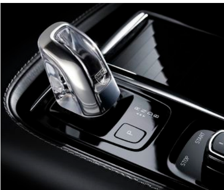
Made from Orrefors® crystal glass, the gear selector in the T8 blends traditional Swedish materials with advanced design and technology.
