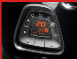
Automatic air conditioning
