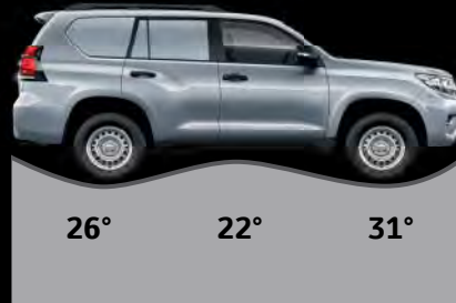
Approach, ramp break-over and departure angles
