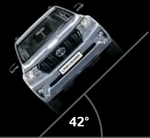
Limit angle of vehicle turnover
