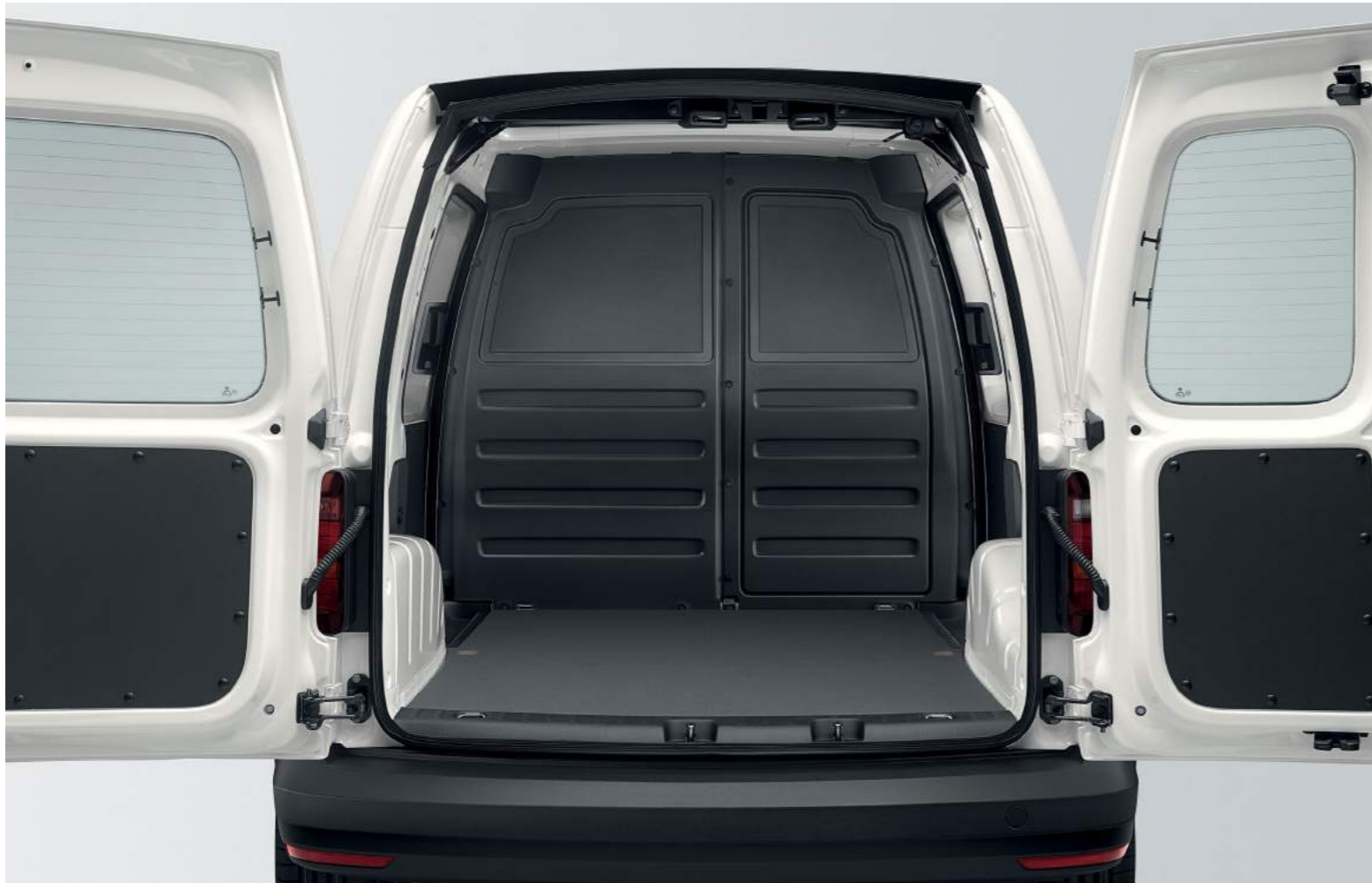
Full-height solid bulkhead. Standard on Caddy Maxi panel van.
