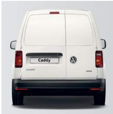
Asymmetric rear wing doors with optional white ABS protective panels.
