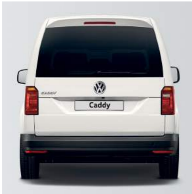
Tailgate with window and spoiler. Standard on Caddy Maxi kombi and optional on panel vans.
