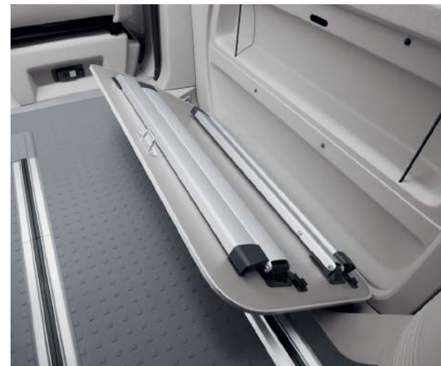
Folding camping table. Conveniently attaches to the inner of the side sliding door.
