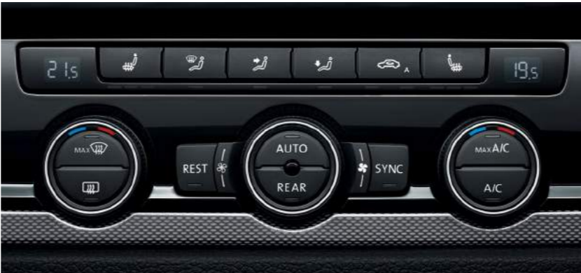
Climatronic three-zone automatic air conditioning and heated seats.
