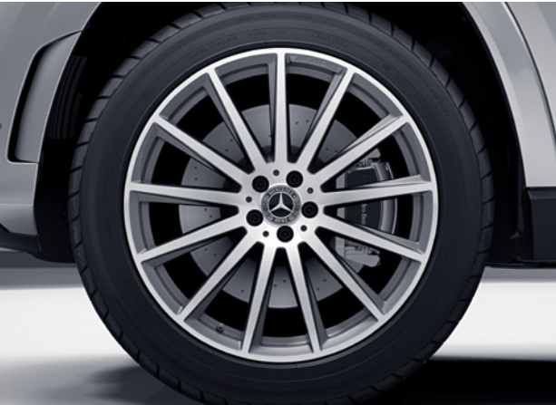
RPA 22" AMG alloy wheels (4) – multi-spoke design, painted titanium grey front: 285/45 tyres; rear: 325/40 tyres
