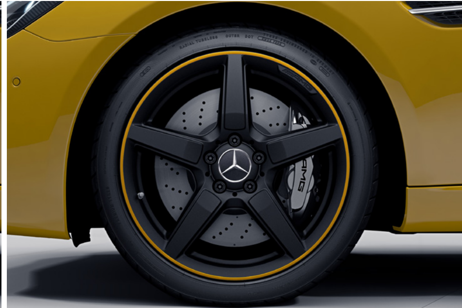
RGK 18" AMG bi-colour alloy wheels (4) – 5-spoke design painted matt black with yellow rim flange front: 235/40 tyres; rear: 255/35 tyres
