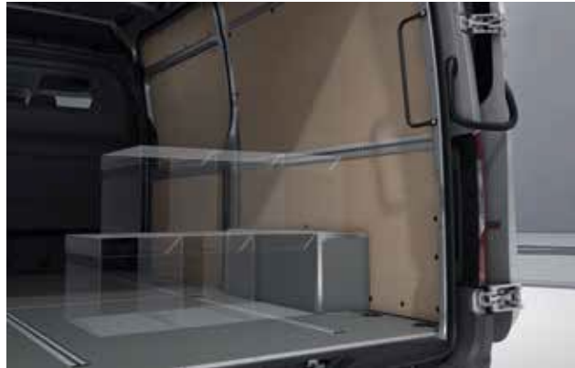
Ply-lining on the wheel arches and van walls from factory makes loading easier and protects the metal panelling from damage.
