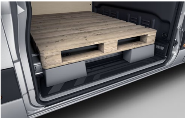
Pallet support in the step of the sliding door stabilises loads in the door area and is particularly useful when transporting Europallets or crates.
