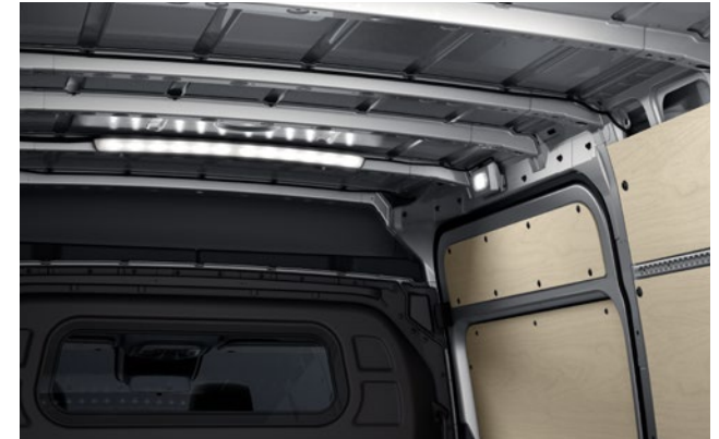
Two LED light strips under the roof illuminate the load compartment, for improved visibility inside when loading and unloading the vehicle.
