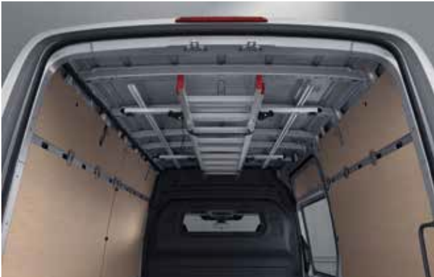
Internally fitted roof racks are available to protect items against theft and prevent the need for external racking to be mounted.
