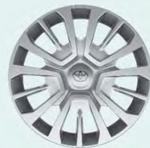
16" steel wheels with wheel caps (5-triple-spoke)
