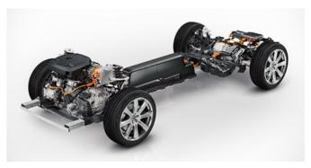
The battery's location helps give your Volvo a low centre of gravity, so it is stable, sure-footed and comfortable while not affecting the car's load space.
