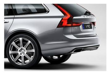
Discover superior comfort and handling with our optional active chassis with rear air suspension. It soaks up poor road surfaces and keeps the ride height constant so the car responds how you want it to. Active chassis technology allows you to customise the way the V90 rides and handles.
