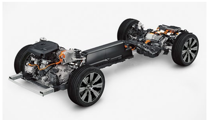
The battery's location helps give your Volvo a low centre of gravity, so it is stable, sure-footed and comfortable while not affecting the car's load space.
