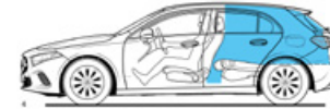
Open luggage compartment behind driver's seat, rear seat backrest folded, loaded to roof, volume 1,125 litres (V 214-1)
