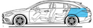
1 Open luggage compartment behind rear seat, loaded to upper edge of rear seat backrest, volume 505 litres (V 211-2)
