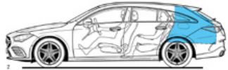
2 Open luggage compartment behind rear seat, loaded to roof, volume 605 litres (V 214-2)
