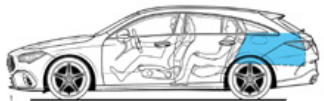
1 Open luggage compartment behind rear seat, loaded to upper edge of rear seat backrest, volume 505 litres (V 211-2)
