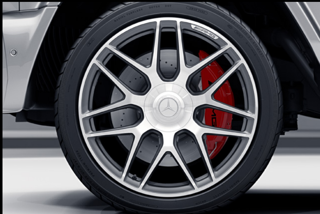
RG5 22" AMG forged wheels – cross-spoke design, painted titanium grey with a high-shine finish, 295/40 R22 tyres
