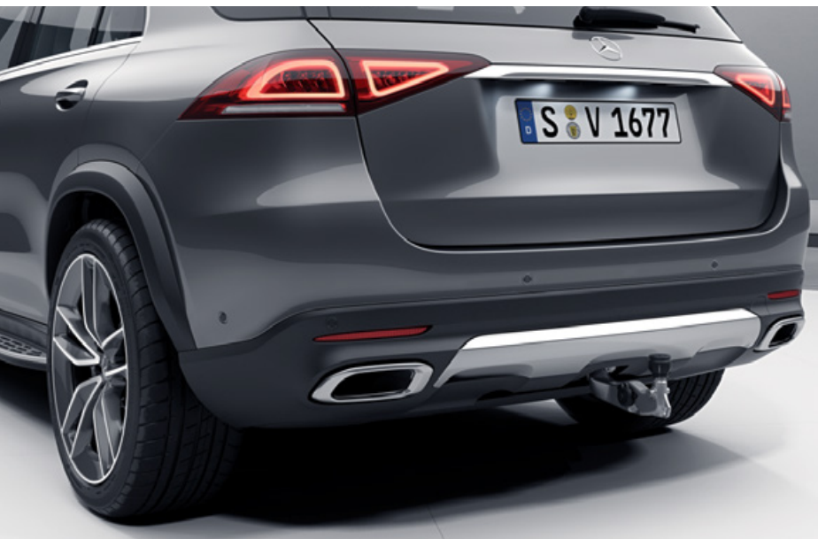
Electronically-folding tow bar (includes 13-pin socket; ESC)
