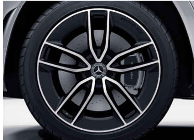
RXT 22" AMG alloy wheels (4) – 5-twin-spoke light-alloy wheels painted in black with a high-sheen finish, front 285/40 tyres; rear: 325/35 tyres
