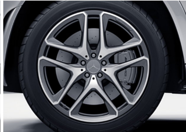
RWD 21" AMG alloy wheels (4) – 5-twin-spoke light-alloy wheels painted in titanium grey with a high-sheen finish, front 275/45 tyres; rear: 315/40 tyres
