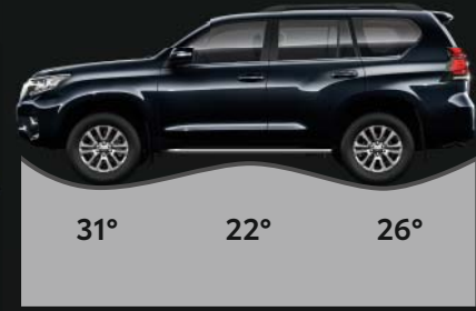
Approach, ramp break-over and departure angles
