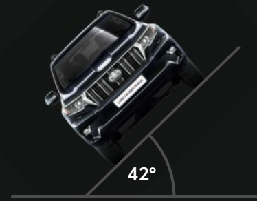
Limit angle of vehicle turnover
