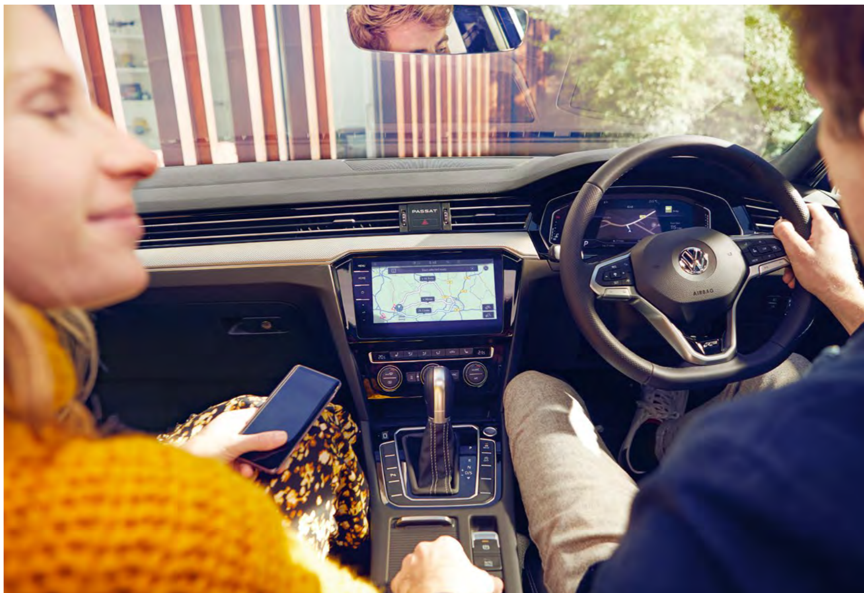
01 The optional Head-up Display 1 presents driving information directly in your field of vision. Speed, traffic signs and information about the assistance systems, as well as warnings and navigation data are projected on to the high-quality retractable screen transparently displayed in front of the windscreen, enabling you to read everything clearly while keeping your focus on the road ahead. Optional on SEL, R-Line, GTE and GTE Advance models.
