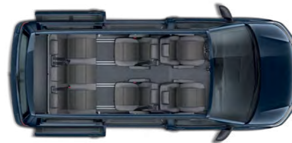
California 6.1 Beach Tour with passenger car registration, two rear sliding doors and 5 seats with 6- or 7-seat options available.
