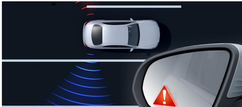
**Active Blind Spot Assist** can warn the driver of vehicles in the blind spot during a lane change and can help to avoid a collision by means of one-sided braking intervention
