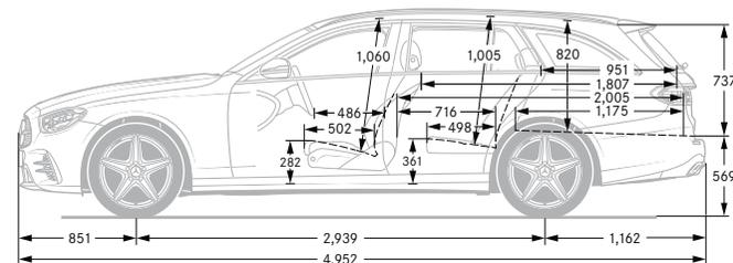
All measurements in millimetres. The dimensions shown are mean values and apply to standard-specification, unladen vehicles
