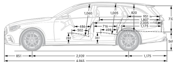
All measurements in millimetres. The dimensions shown are mean values and apply to standard-specification, unladen vehicles
