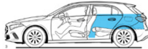
3 Open luggage compartment behind driver's seat, rear seat backrest folded, loaded to upper edge of driver's backrest, volume 780 litres (V 211-1)
