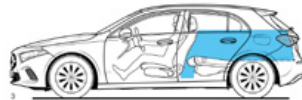
3 Open luggage compartment behind driver's seat, rear seat backrest folded, loaded to upper edge of driver's backrest, volume 825 litres (V 211-1)
