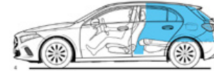
4 Open luggage compartment behind driver's seat, rear seat backrest folded, loaded to roof, volume 1,125 litres (V 214-1)
