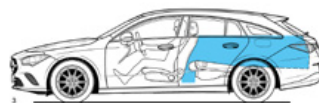
Open luggage compartment behind driver's seat, rear seat backrest folded, loaded to upper edge of driver's backrest, volume 960 litres (V 211-1)
