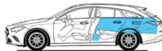
Open luggage compartment behind driver's seat, rear seat backrest folded, loaded to upper edge of driver's backrest, volume 900 litres (V 211-1)
