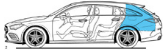
2 Open luggage compartment behind rear seat, loaded to roof, volume 605 litres (V 214-2)
