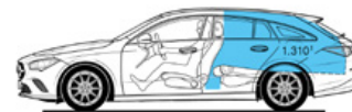
Open luggage compartment behind driver's seat, rear seat backrest folded, loaded to roof, volume 1,310 litres (V 214-1)
