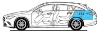
Open luggage compartment behind rear seat, loaded to upper edge of rear seat backrest, volume 454 litres (V 211-2)
