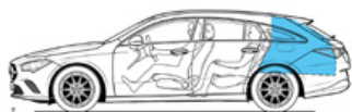
Open luggage compartment behind rear seat, loaded to roof, volume 605 litres (V 214-2)
