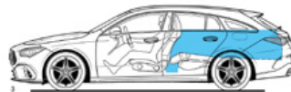
3 Open luggage compartment behind driver's seat, rear seat backrest folded, loaded to upper edge of driver's backrest, volume 960 litres (V 211-1)
