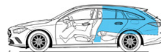
Open luggage compartment behind driver's seat, rear seat backrest folded, loaded to roof, volume 1,370 litres (V 214-1)
