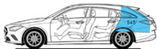
Open luggage compartment behind rear seat, loaded to roof, volume 545 litres (V 214-2)
