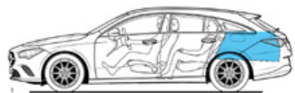
Open luggage compartment behind rear seat, loaded to upper edge of rear seat backrest, volume 505 litres (V 211-2)
