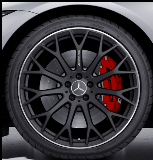
RWG 21" AMG alloy wheels – multi-spoke design, painted matt black with a high-shine finish rim flange
