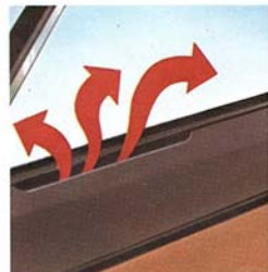
The ventilation system is complemented by two air inlets in the doors for side window demisting.
