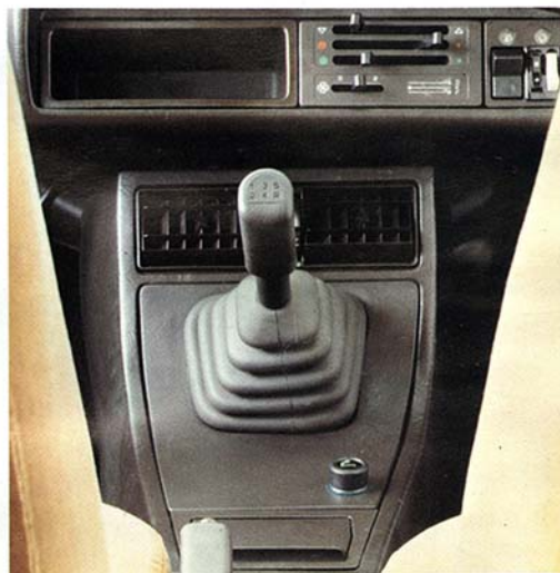
The five speed gearbox is standard and the centre console incorporates an illuminated ashtray and cigarette lighter.
