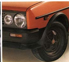
The front spoiler increases front end adhesion at high speeds.
