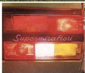
Rear light cluster incorporating fog warning light.
