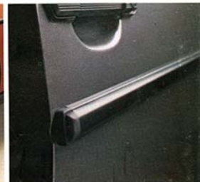
Matt black side rubbing strips offer protection from minor impacts.
