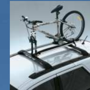
> Bike Carrier. Sturdy lockable alloy carrier secures a bike in an upright position.
