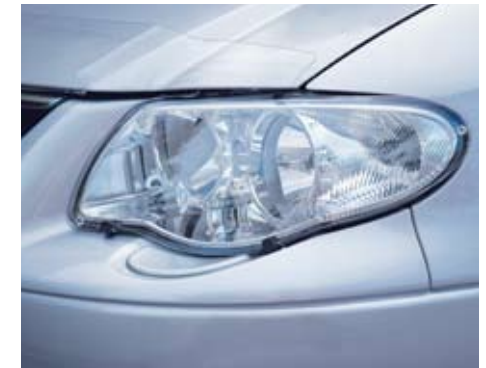
HEADLIGHT PROTECTORS help to prevent damage to headlamps caused by loose stones or road debris.
