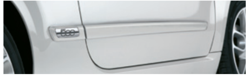
Side mouldings with space for badge* Part No 5090I675
