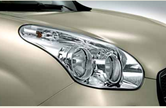
The characteristic, three-dimensional, wrap-around headlights stretch back at the top to incorporate the indicators.
