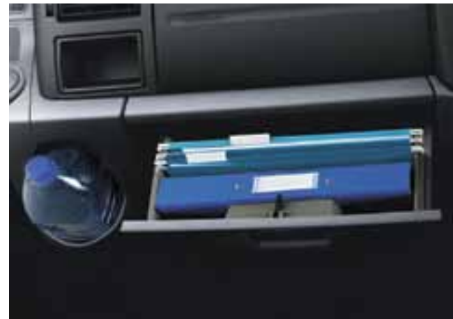
Clever ideas include rails in the larger than normal glovebox so you can hang A4 files.
