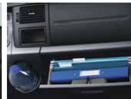
Clever ideas include rails in the larger than normal glovebox so you can hang A4 files and storage for two 2-litre bottles.
