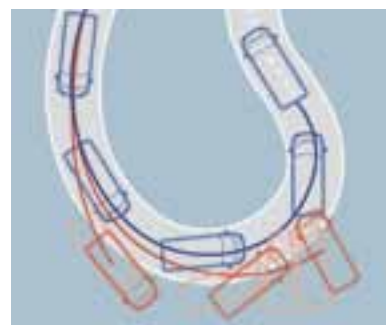
Dynamic Stability Control (DSC) helps avoid understeering and oversteering by correcting the driving line through a combination of brake application to the appropriate wheel and a reduction in engine torque.
