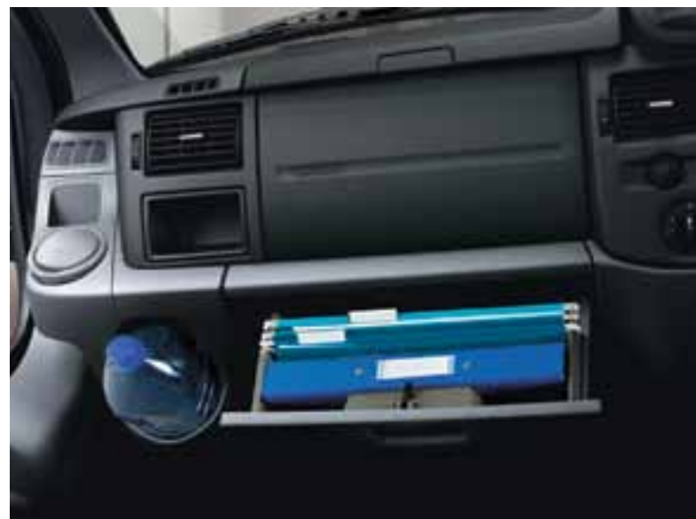
Clever ideas include rails in the larger than normal glovebox so you can hang A4 files.
