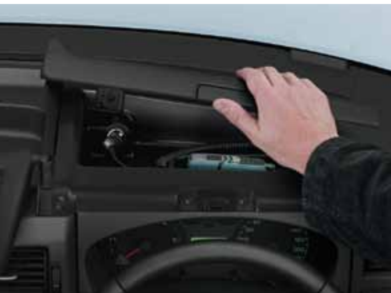
One of the two lidded storage compartments on the dashboard is fitted with a 12-volt power socket so you can discreetly charge a mobile phone away from prying eyes.
