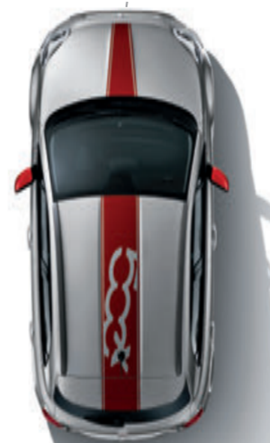
DECALS ON BONNET AND ROOF IN RED COLOUR With 500X logo. Not compatible with sunroof version (opt. 400). REF. 50927498
