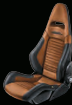
Natural leather/Alcantara® Sabelt seats with carbon fibre shell
