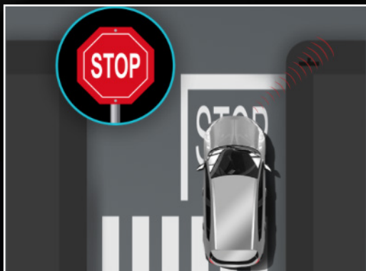
Traffic Sign Recognition: displays traffic signs and speed limits on the TFT instrument display
