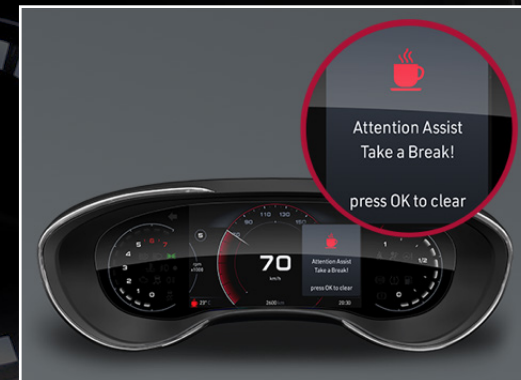
Attention Assist: the system detects and warns against signs of driver fatigue with an audible warning
