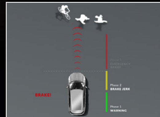
Autonomous Emergency Braking: helps to mitigate against frontal collisions
