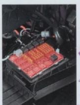
The power distribution box, ahead of the main fusing system, provides added under-hood electri-
