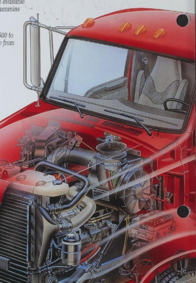
•Extensive use of straight radiator hose and tubing permits readily available stock material to be used for most repairs.
