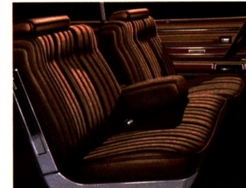
Saddle Oxen- and Madrid-grain expanded vinyl 60/40 notchback seat, available in Electra Limited Hardtop Coupe and Sedan. Saddle only.
